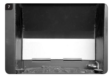
4.7 With the liners and baffle removed the firebox is clear for cleaning and maintenance, see Diagram 8.
