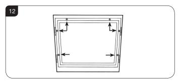
7.10 Replace ALL of the securing screws ensuring that a screw is present in all fixing slots.
