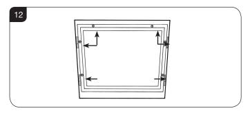
8.3 Replace ALL of the securing screws ensuring that a screw is present in all fixing slots.
