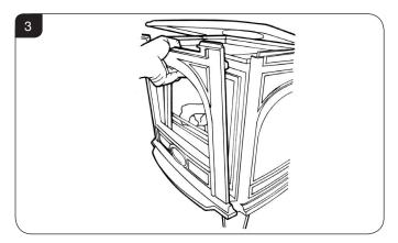
5.4 Remove the glass frame by undoing the fixing screws and lifting clear, see Diagram 4. Take care to support the glass window panel when removing the screws.
