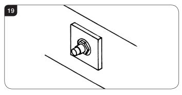
11.5 Extract the injector with the feed pipe from beneath the appliance.
