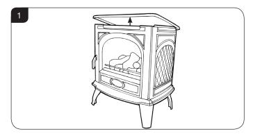
Lift the front upwards until it is clear of the slots and pull away from the appliance, see Diagram 2.
