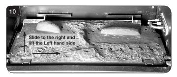
5.4 Slide the burner back to the left and out of its location.
