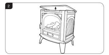
5.4 Lift the front upwards until it is clear of the slots and pull away from the appliance, see Diagram 3.
